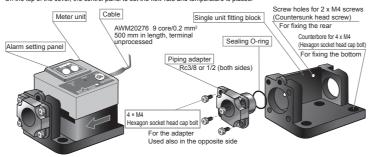
Note: For the single unit fitting block, it is possible to fix its bottom (by using four M4 hexagon socket head cap bolts), to fix its rear (by using two M4 countersunk head screws), or to fix with a pipe, depending on the mounting dimensions.
